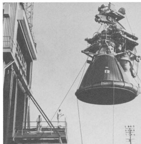
F-1 engine is placed in test stand at Marshall Center test area.
