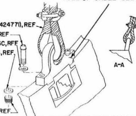
FIG. 3. INSTALLING BUMPERS AND CABLE ASSEMBLIES
