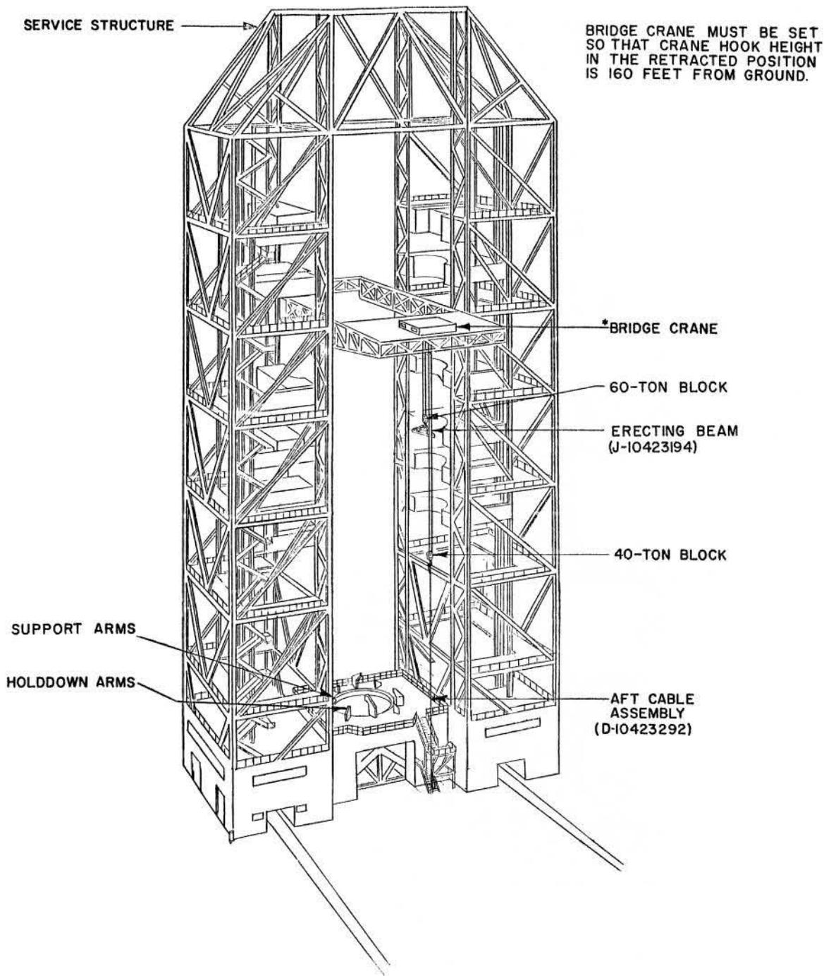
FIG. 17. PREPARING SERVICE STRUCTURE FOR ERECTION
