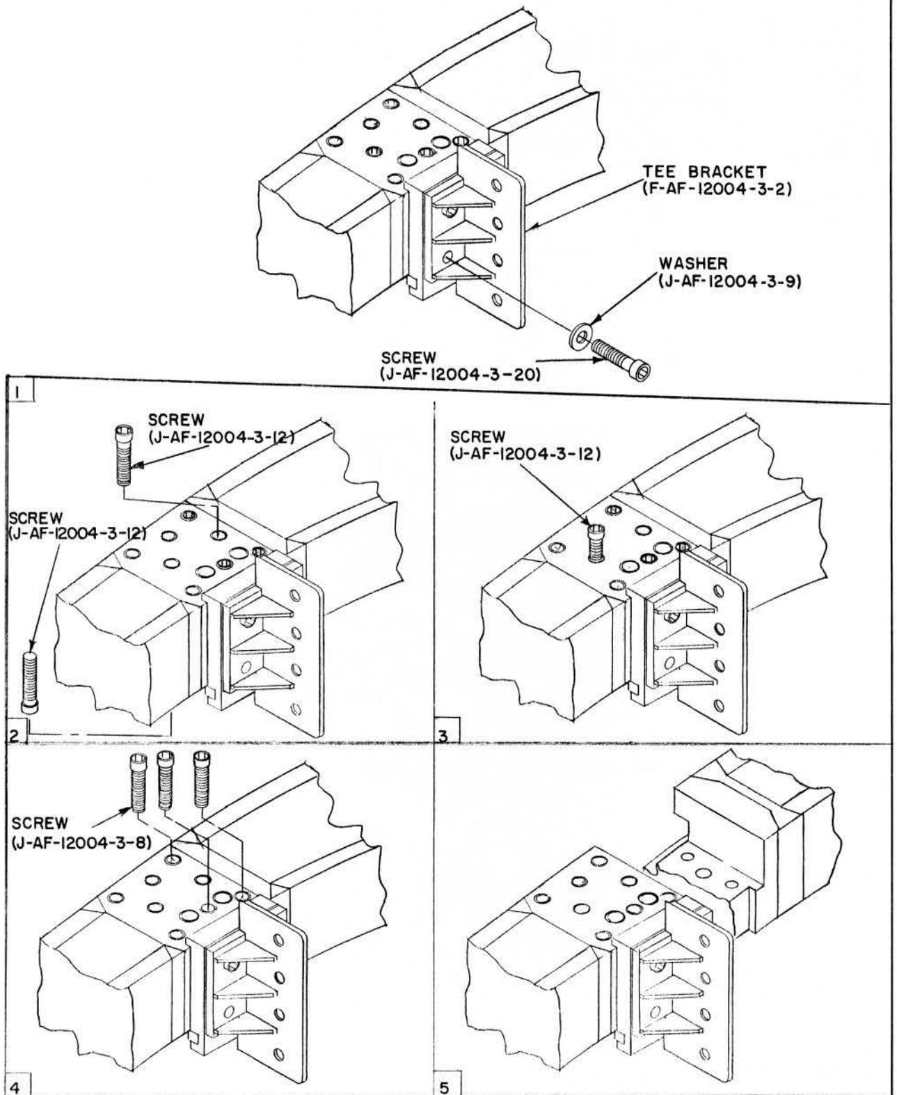
FIG. 23. FORWARD RING SECTION REMOVAL PROCEDURES
