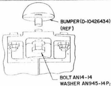
INSTALL LUG IN LINE OF PULL OF CABLE-SEE A-A
