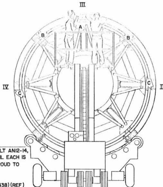
AFTER BUMPER IS SECURED BY BOLT ANI2-14, UNSCREW BOTH BOLTS (AN8-6A) UNTIL EACH IS SEATED AGAINST BOLT HOLDING SHROUD TO BRACKET.
