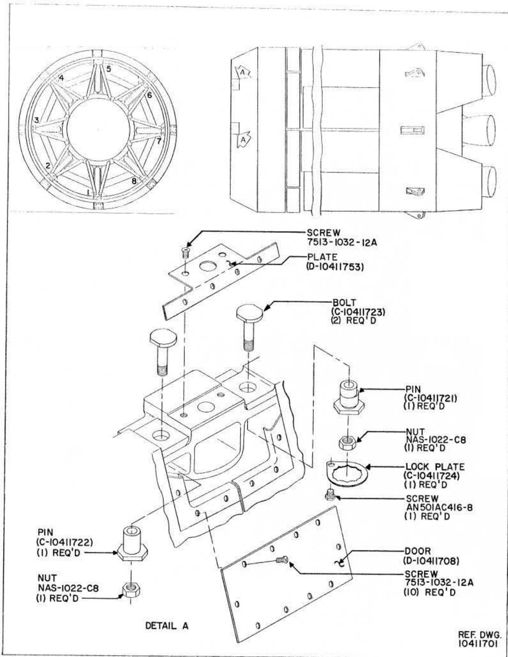
FIG.2 REMOVING DOORS AND PLATES
