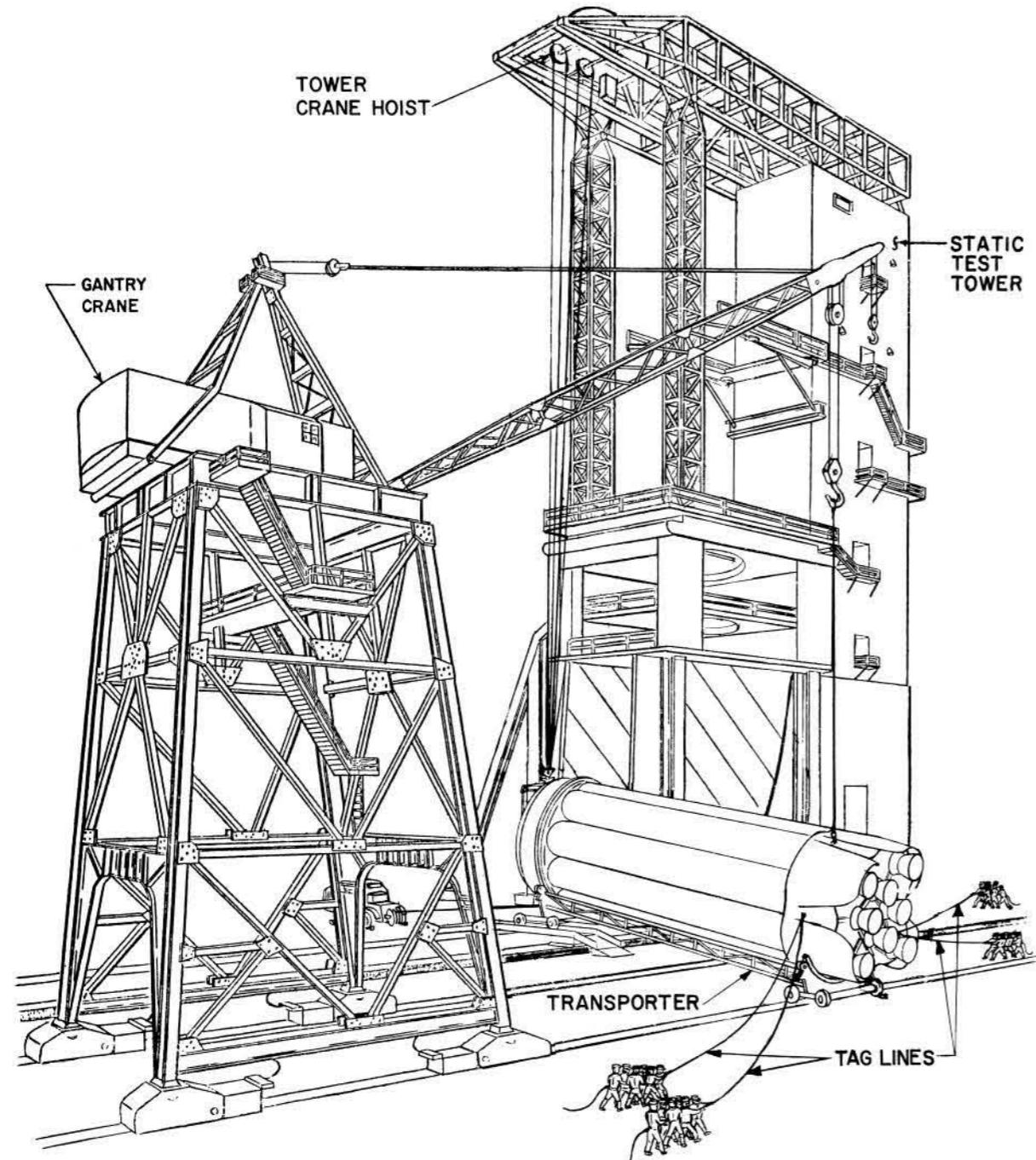
PRIOR TO LIFTING THE BOOSTER FROM THE TRANSPORTER STABILIZE THE BOOSTER SO THAT THE PIN THROUGH OUTRIGGER NO.1 IS FLOATING IN THE RECESS OF TEE BRACKET.
