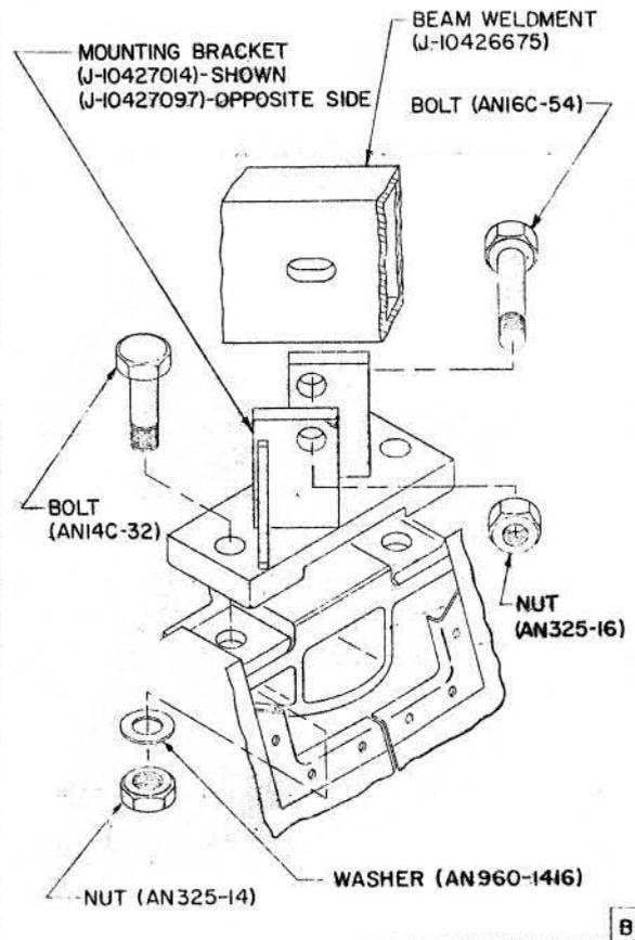
FIG. 20. INSTALLATION OF BEAM WELDMENT AND FOWARD SLING ASSEMBLIES
