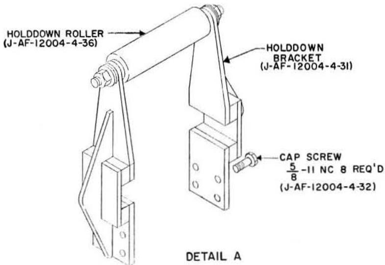
FIG.12 FORWARD SUPPORT CLAMPS
