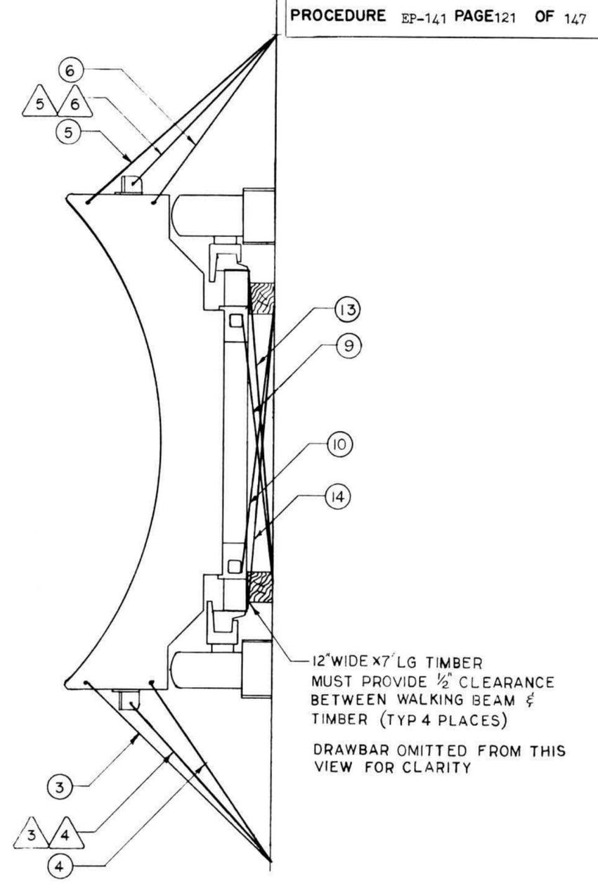
FIG. 46. TIE-DOWN ARRANGEMENT S-1 TO BARGE
