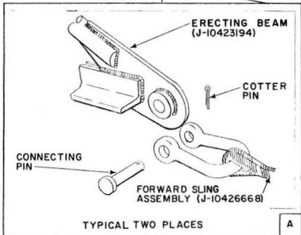
FIG. 25. CONNECTING ERECTING BEAM AND FORWARD SLING ASSEMBLIES
