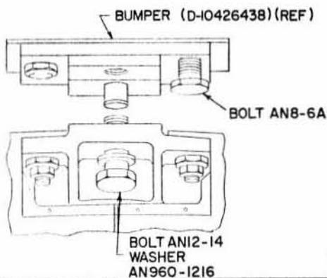
NOTE: WHENEVER CABLE ASSEMBLY (10424771) IS ATTACHED, NEW BOLTS, WASHER, AND NUTS SHALL BE INSTALLED, USED HARDWARE TO BE DISCARDED.
