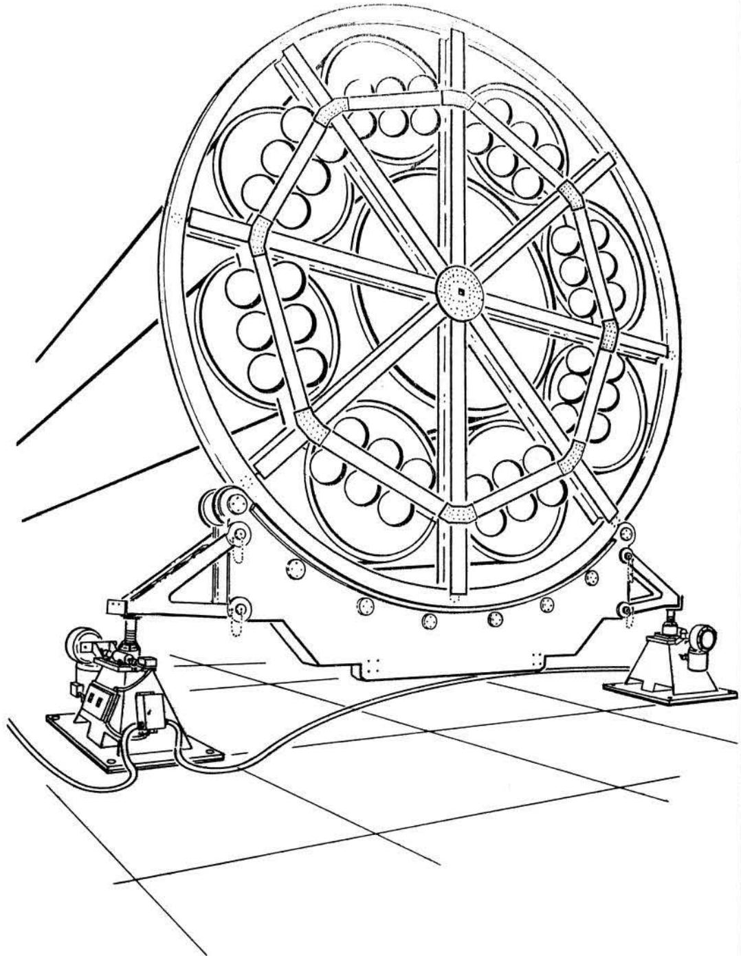
FIG. 52 FIXTURE ASSEMBLY SUPPORTED BY JACK ASSEMBLIES
