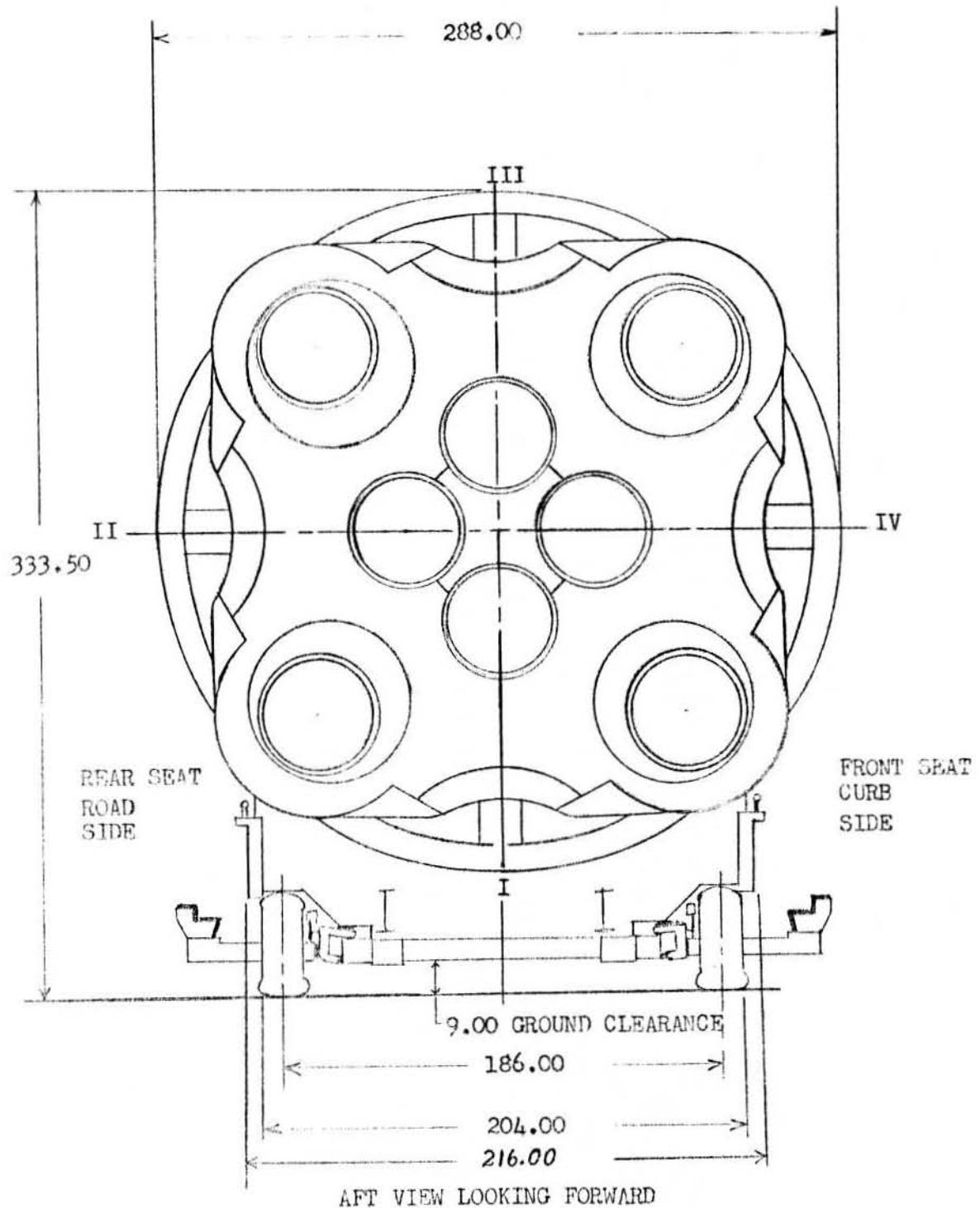
FIG. 33. SATURN TRANSPORTER DEMENSIONS (SHEET 2 OF 2)
