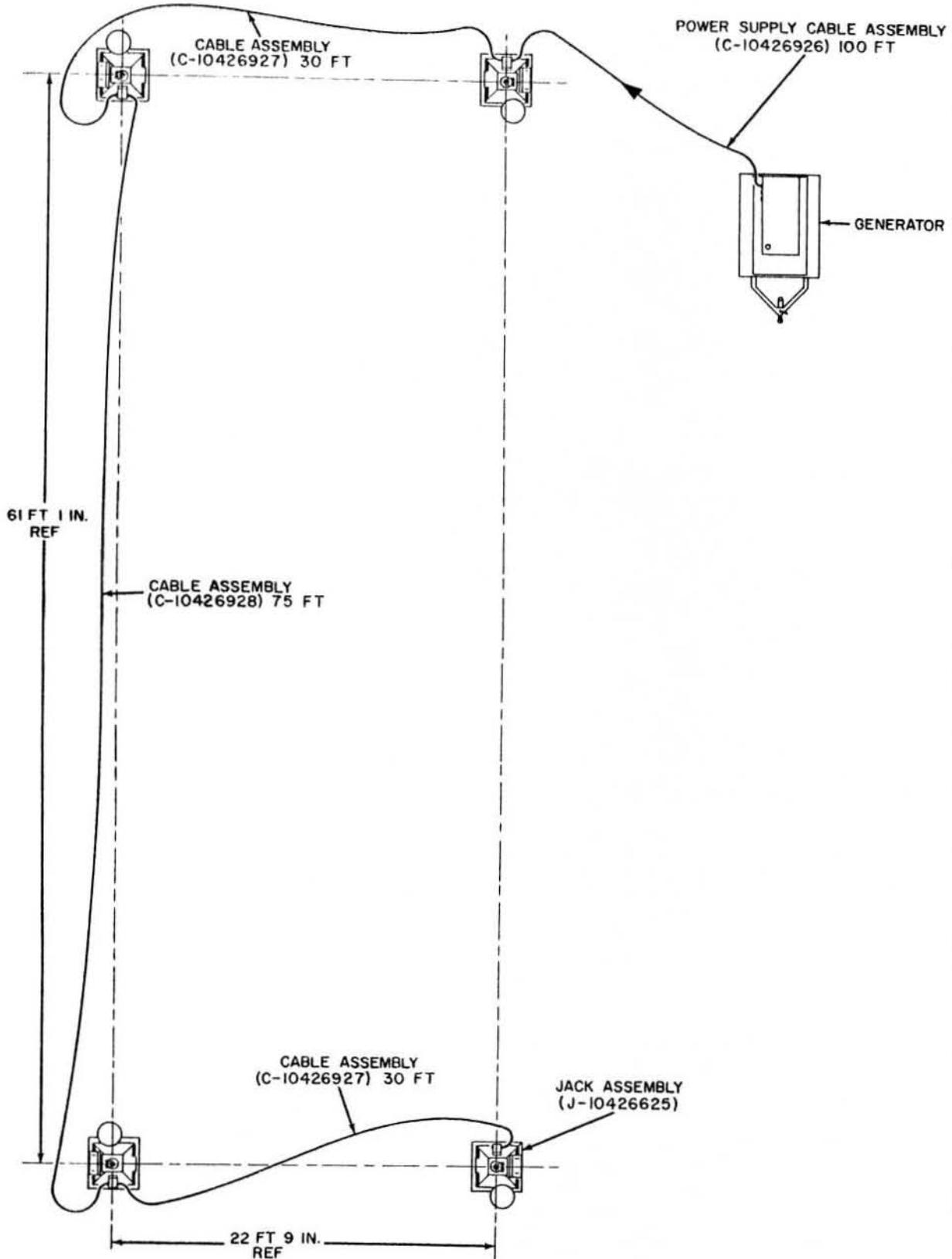
FIG. 48 JACK POSITIONING AND CABLE INTER-CONNECT DIAGRAM
