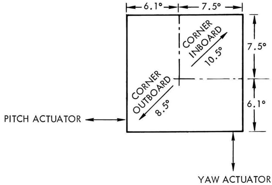
The servoactuators are compatible with the engine alignment requirement of 0 degrees 27 minutes. They incorporate an effective piston area of 13.0 square inches, a dual element potentiometer, a locking device that actuates upon loss of hydraulic pressure, and a cylinder bypass valve for both manual and remote operation. The main hydraulic pump incorporates a thermal barrier to isolate the pump from the LOX turbine environment.
