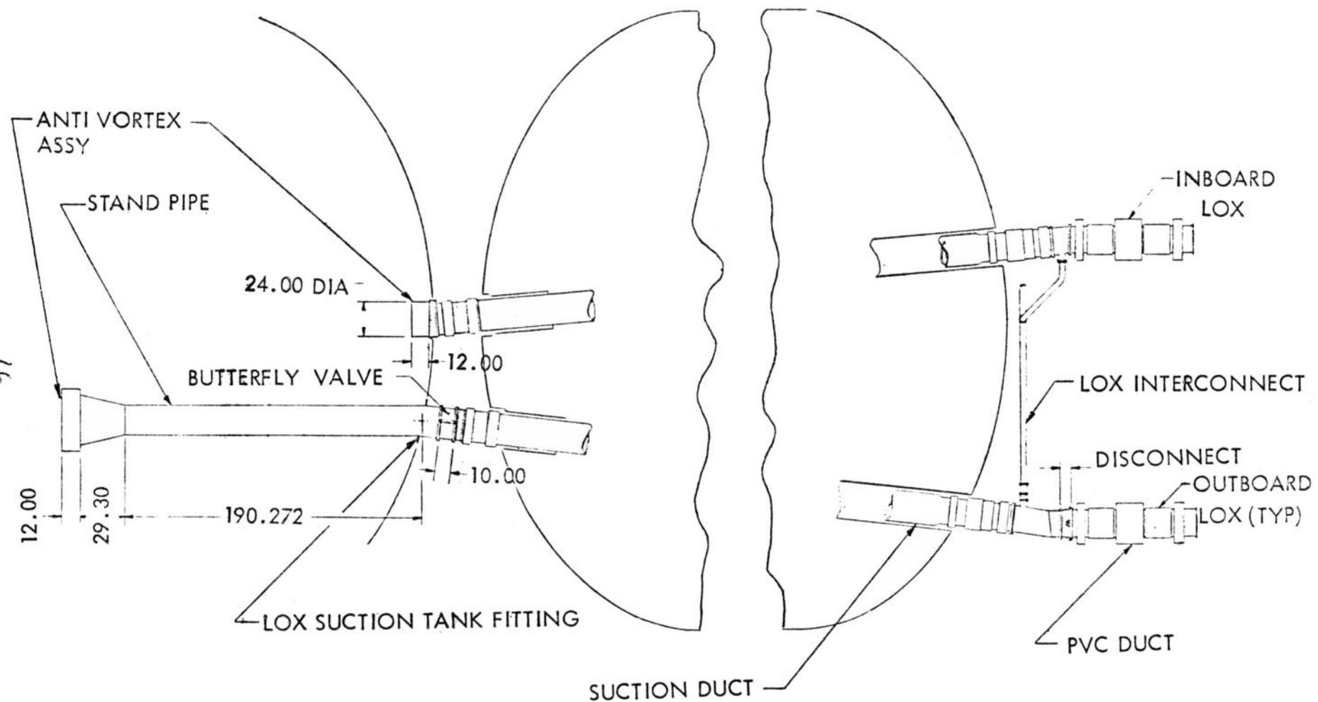
THRUST STRUCTURE LOX DELIVERY SYSTEM
