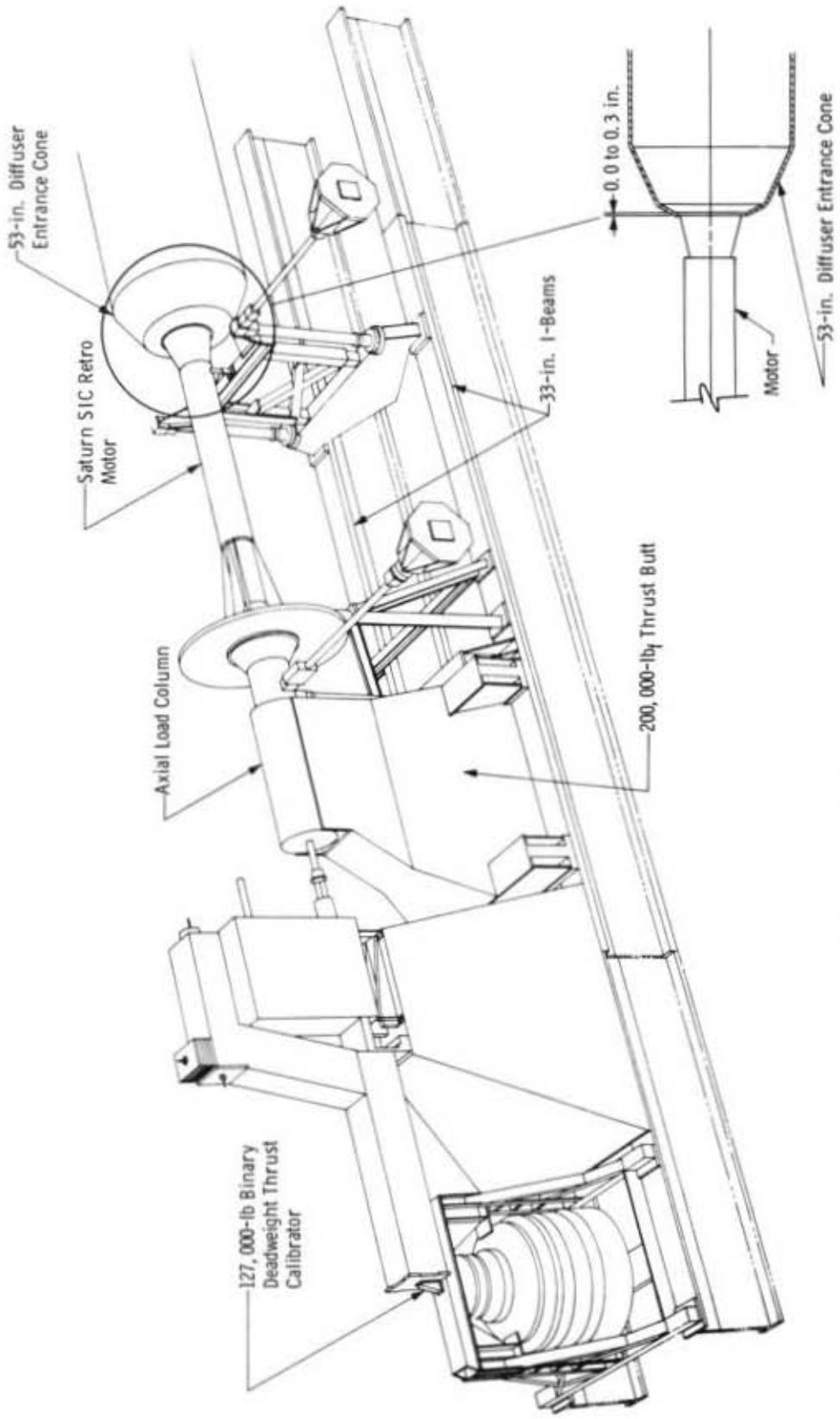
d. Schematic of Thrust Measuring System
