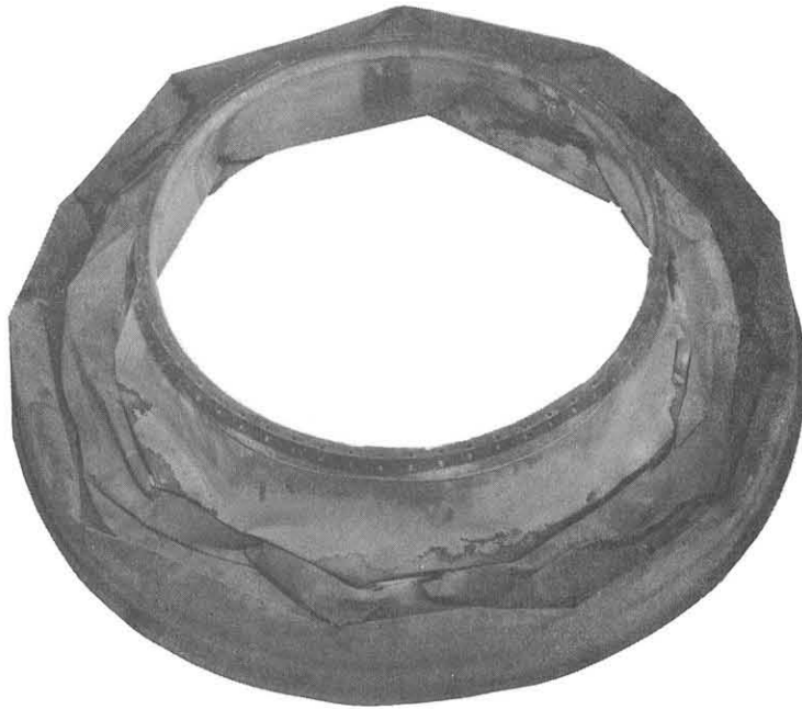
Figure 17. Columbia Nozzle Extension After Crushing Test
