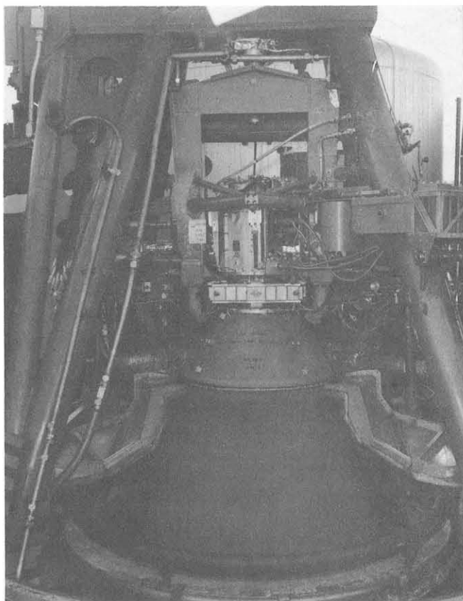
Figure 24. LMDE Installed in High Altitude Test Stand
