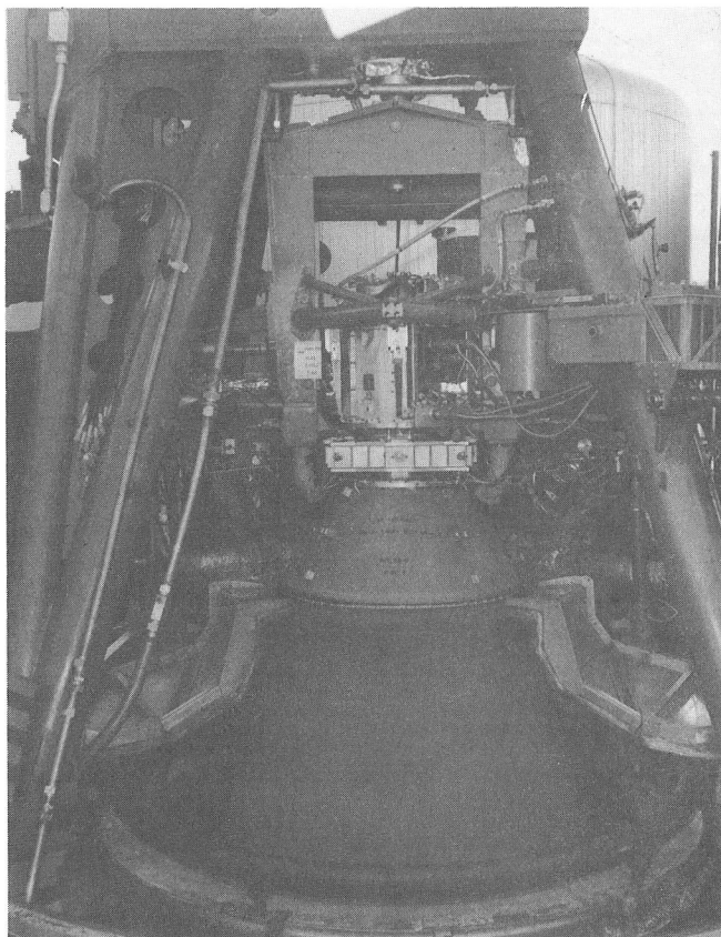
Figure 24. LMDE Installed in High Altitude Test Stand
