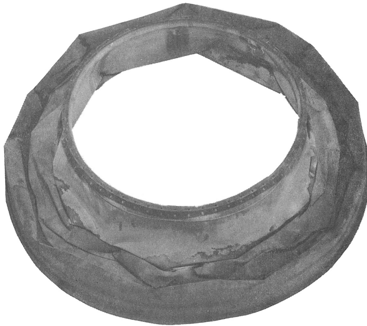
Figure 17. Columbia Nozzle Extension After Crushing Test
