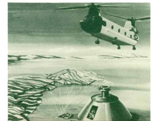
The blunt end of the command module heats up like a fireball. Pressure and friction of the atmosphere and then a drogue chute slow the module, and at 10,000 feet the main parachutes open to bring it to a safe ground landing. Radar and optical instruments track its descent, and helicopter recovery teams proceed immediately to pick up the three crewmen.
