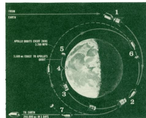
On the next trip around, if everything is all right, the lunar excursion vehicle will land. A large glass area allows the two astronauts to have a clear view of the touchdown site. With retrorocket firing and legs extended, the vehicle descends to within 100 feet of the lunar surface. The vehicle will be able to hover for almost a minute or move laterally for about 1,000 feet for choosing the best touchdown point.
