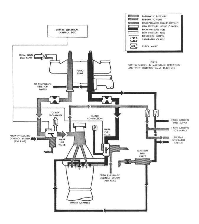
Propellant Subsystem Data Flow
