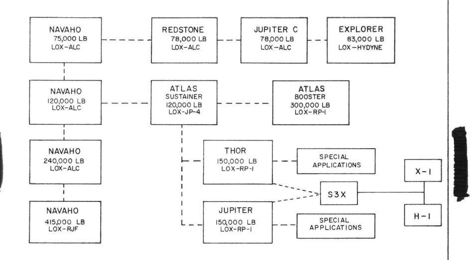
Figure 1. Family Tree of Rocketdyne Engines
