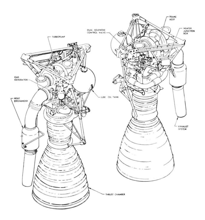
Figure 2. S-3D (JUPITER) Rocket Engine
