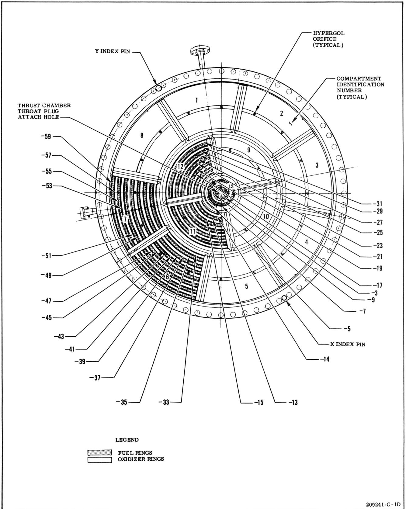
Figure 1-24. (C) Thrust Chamber Injector--Cutaway View (Sheet 2 of 2)
