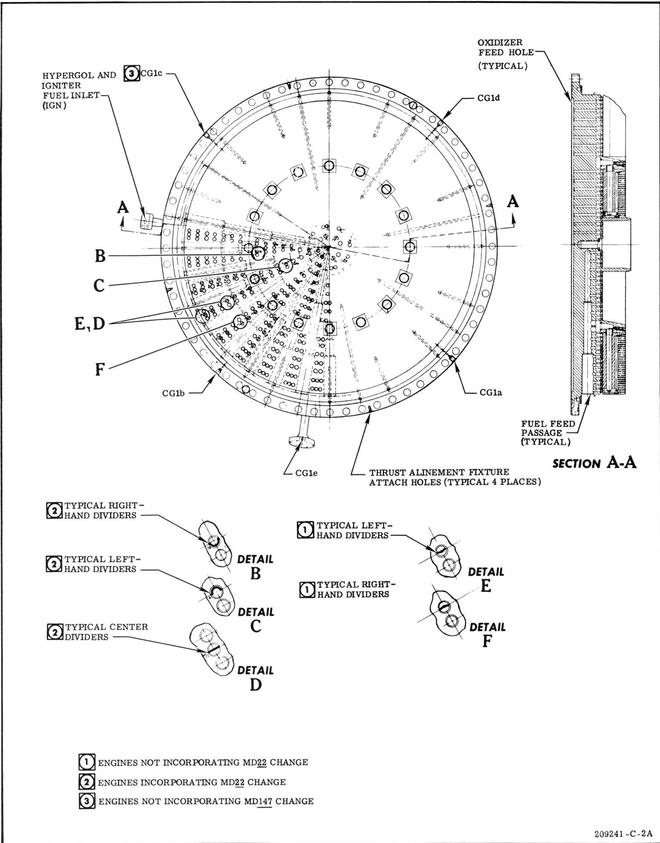
Figure 1-24. (C) Thrust Chamber Injector--Cutaway View (Sheet 1 of 2)
