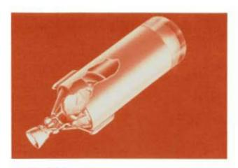
The S-IVB will measure about 22 feet in diameter and about 58 feet in length. Its one J-2 engine can be moved freely in any direction for pitch and yaw control. Propellant capacity of the stage will be 230,000 pounds, which is consumed in just over seven minutes.
