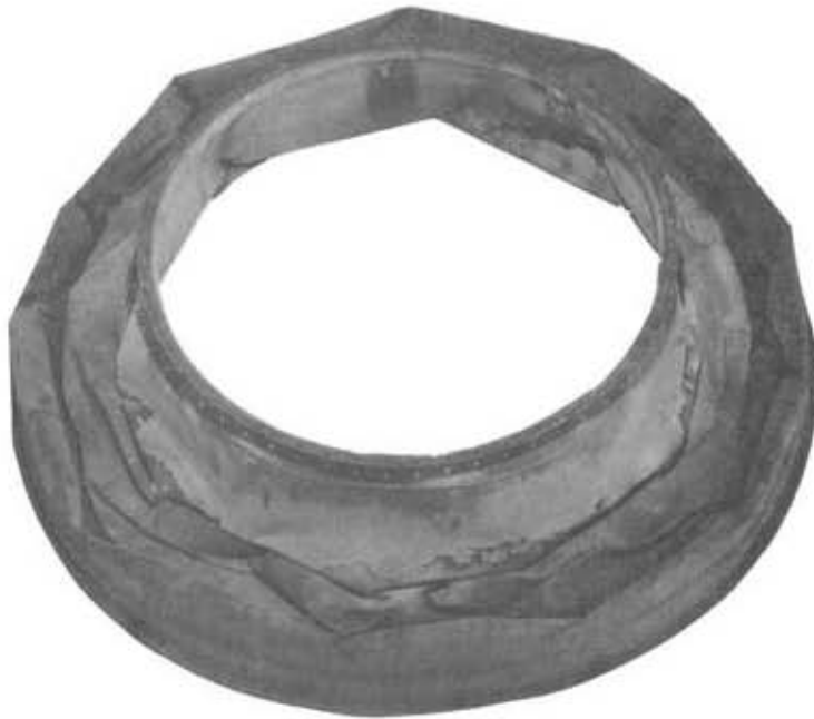
Figure 17. Columbia Nozzle Extension After Crushing Test
