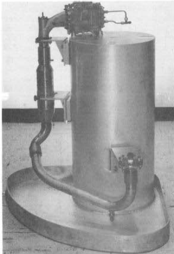
Figure 22. Component Test of Inlet Lines, Flow Control Valve and Shutoff Valve
