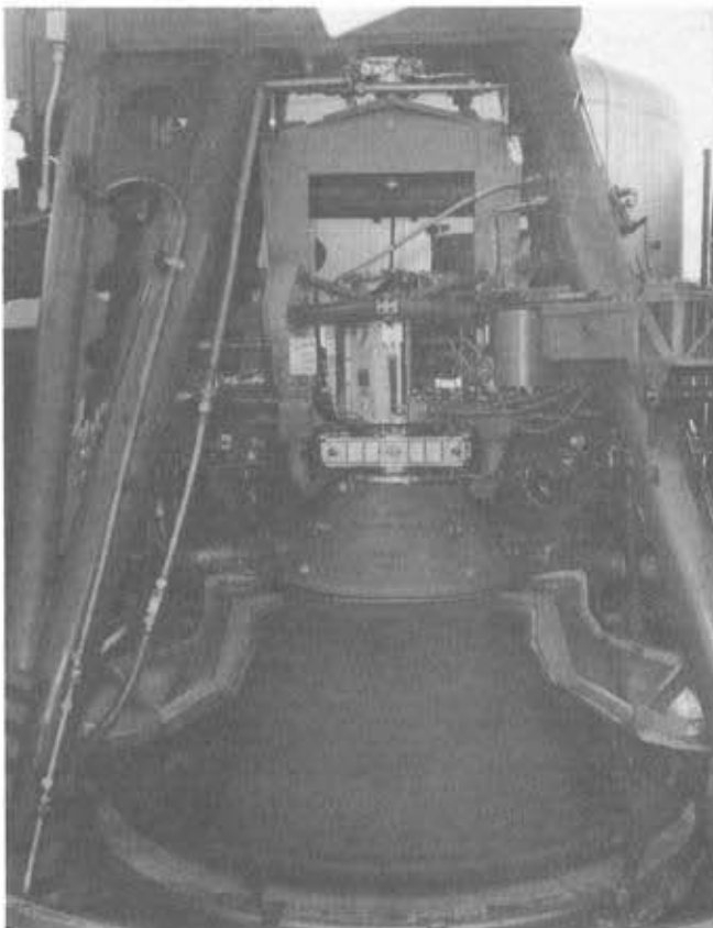
Figure 24. LMDE Installed in High Altitude Test Stand
